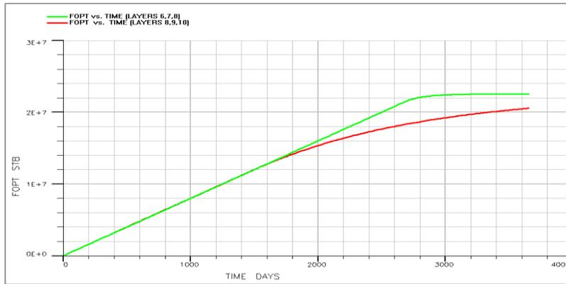
**Fig. 8. Considering the effect of location of created hydraulic fractures on the cumulative oil production in the studied reservoir**
