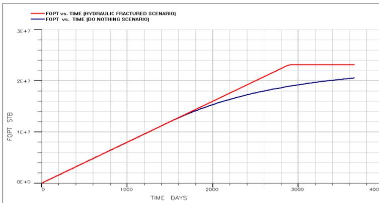
**Fig. 10. Considering the production with and without hydraulic fracturing in “Z” reservoir.**
