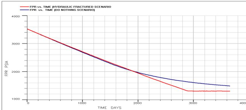
**Fig. 11. Considering the pressure drop with and without hydraulic fracturing in “Z” reservoir.**
