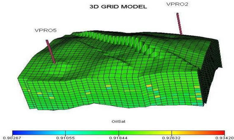
**Fig. 1. Three-dimensional structure of “Z” oil reservoir in southern Iran with two producing fractured wells.**
