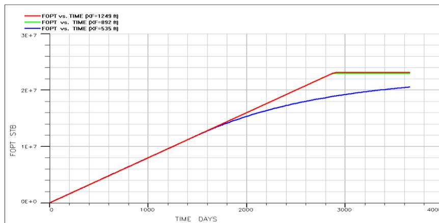
Fig. 6. Considering the effect of fracture length on the cumulative oil production in reservoir “Z”.
