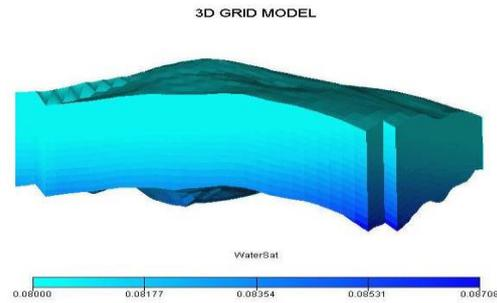
**Fig. 2. Distribution of water saturation in three-dimensional structure of “z” oil reservoir in southern Iran.**
