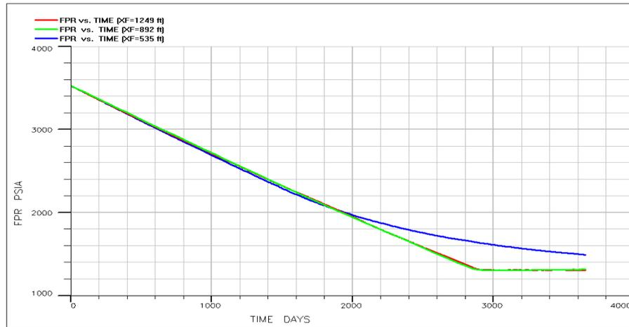
**Fig. 7. Considering the effect of fracture length on the pressure drop in reservoir “Z”.**
