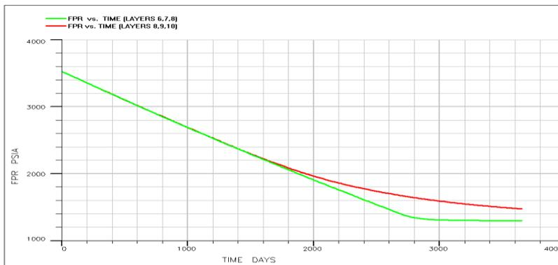
**Fig. 9. Considering the effect of hydraulic fractures location on the pressure drop in the studied reservoir.**
