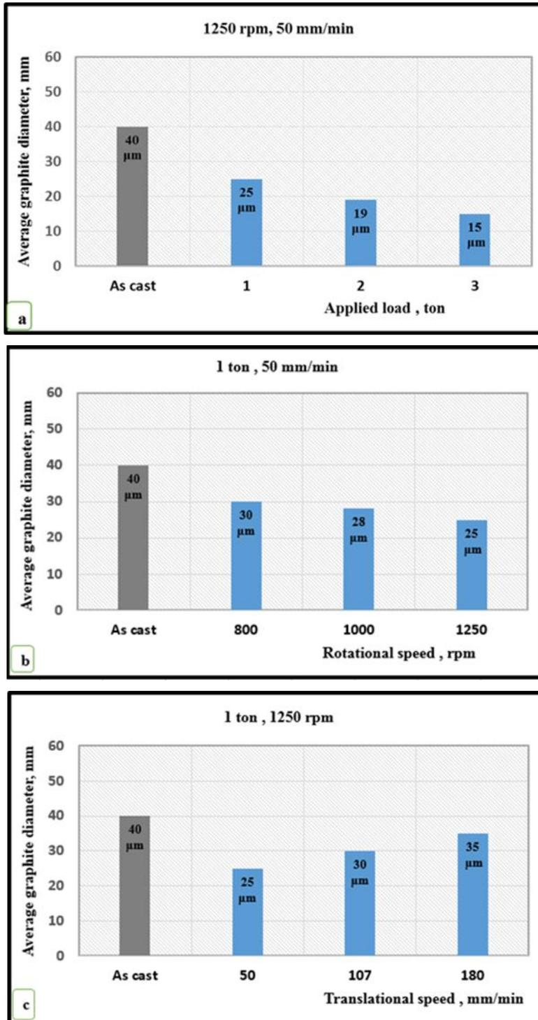
Fig. 5. Average graphite diameter in PZ with various process parameters: (a) applied load (b) rotational speed and (c) translational speed.
