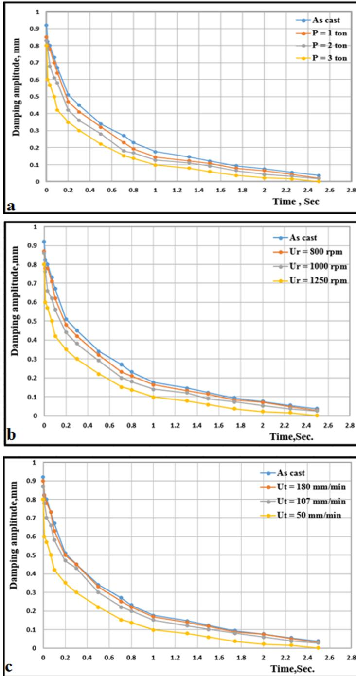
Fig. 9. Decay profiles (time domain) for FSP specimen with varied process parameters: (a) applied load, (b) rotational speed, (c) translational speed.
