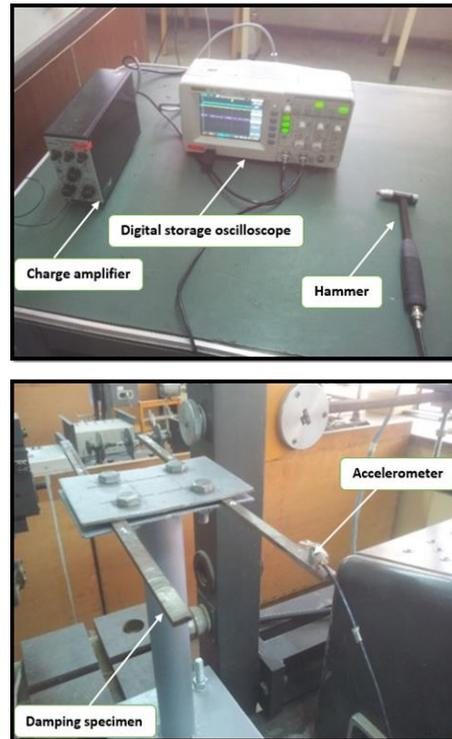
**Fig. 3. Damping test experimental setup.**
