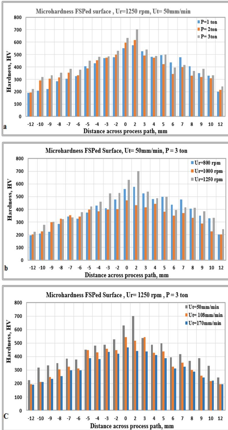
Fig. 6. Hardness variation across process path with process parameters: (a) applied load (b) rotational speed and (c) translational speed.
