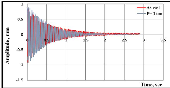
**Fig. 7. Decay signal (time domain) for as cast and FSP specimen with 1 ton, 1250 rpm and 50 mm/min.**
