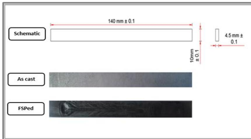
**Fig. 2. Damping test specimen.**
