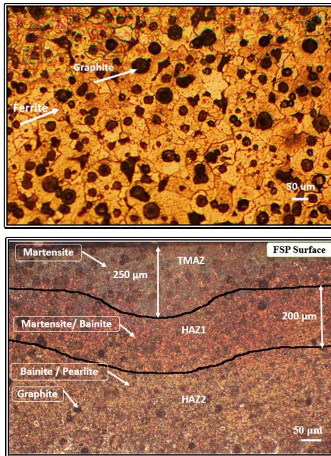
**Fig. 4.** As cast and FSP microstructure with different zones across thickness zones at 3 ton, 1250 rpm, 50 mm/min.
