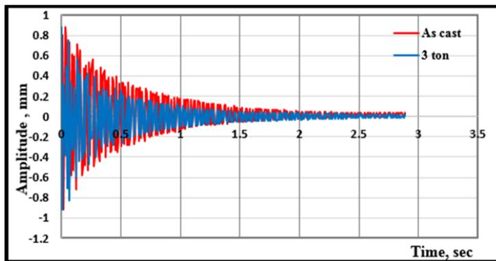
**Fig. 8. Decay signal (time domain) for as cast and FSP specimen with 3 ton, 1250 rpm and 50 mm/min.**
