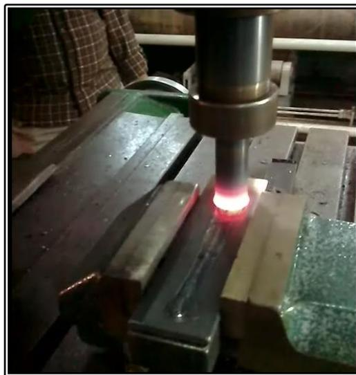
**Fig. 1. Vertical Milling machine type DECKEL, FP4M used for FSP of ferritic nodular cast iron specimens.**
