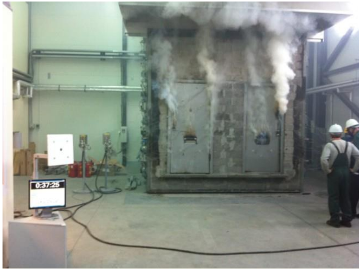
Fig. 3. View of the furnace during the fire test.
