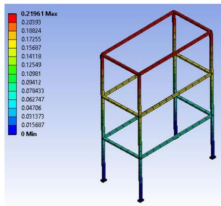
(c). Deformation of base isolated building with RTI at 15 s.
