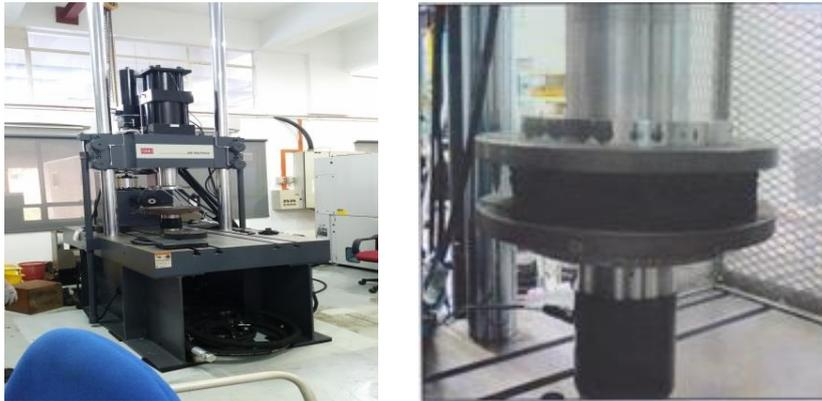
**(a) Servo Hydraulic MTS322. (b) Sample under compression.**
