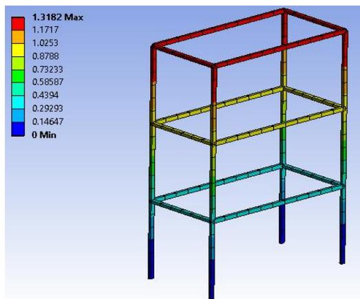
(c). Deformation of fixed base building at 15 s.
