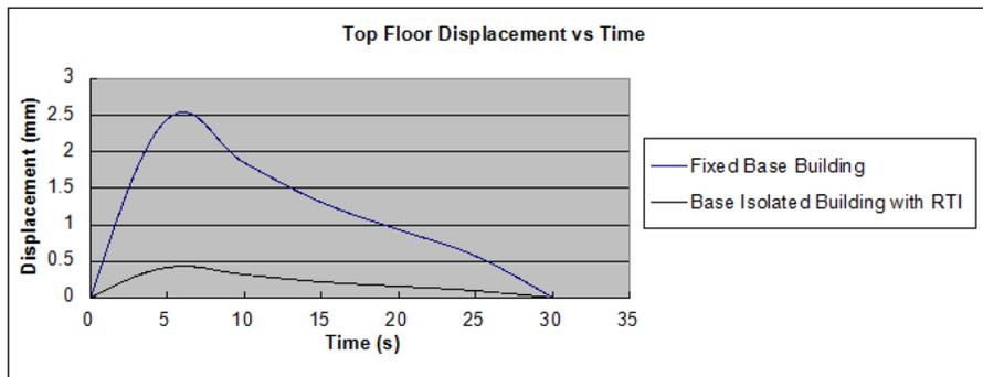
**Fig. 6. Comparison of top floor displacement between fixed base and base isolated building with RTI.**
