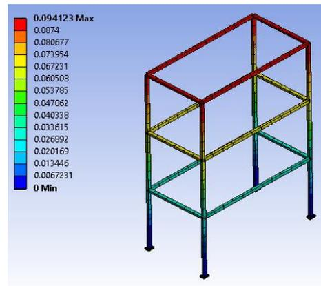
(e). Deformation of base isolated building with RTI at 25 s.
