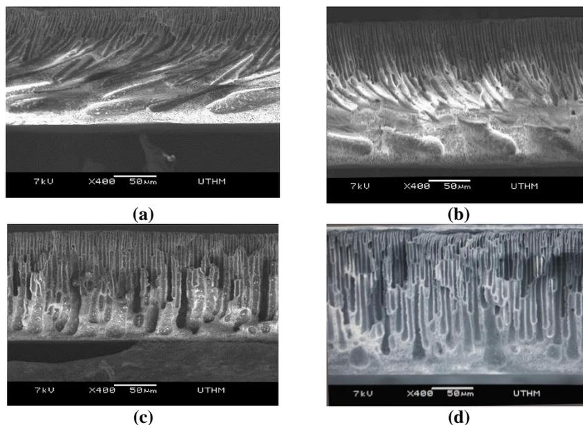
**Fig. 1. SEM cross sectional images of PSF membrane made of different additives at different loading, (a) 7 wt.% PEG (Run 1), (b) 5 wt.% zinc oxide (Run 4), (c) 5 wt.% eugenol (Run 8) and (d) 5 wt.% zinc oxide and 5 wt.% eugenol (Run 10).**
