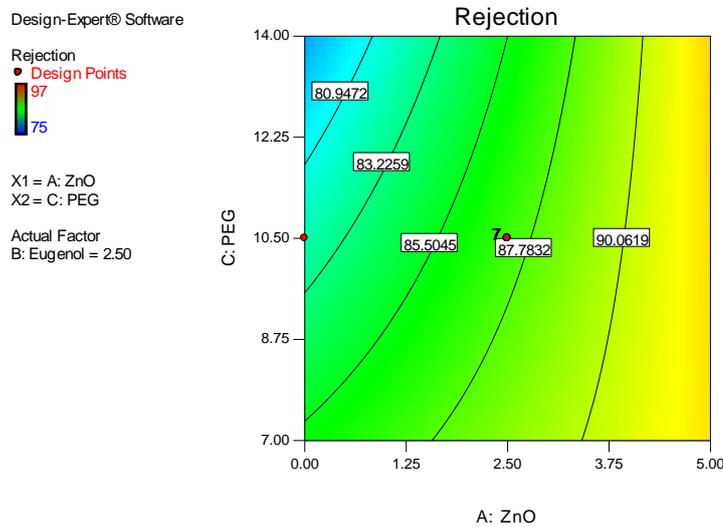
**Fig. 7. Contour plot for interaction between zinc oxide and PEG on membrane rejection.**
