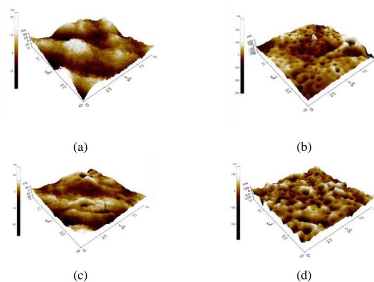
**Fig. 2. Surface roughness of PSF membrane made of different additives at different loading, (a) 7 wt.% PEG (Run 1) ( $R_a$ : 15.70 nm), (b) 5 wt.% zinc oxide (Run 4) ( $R_a$ : 36.25 nm), (c) 5 wt.% eugenol (Run 8) ( $R_a$ : 10.55 nm) and (d) 5 wt.% zinc oxide and 5 wt.% eugenol (Run 10) ( $R_a$ : 31.16 nm).**
