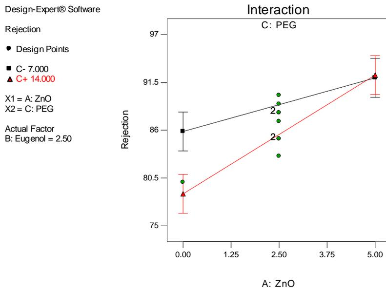
**Fig. 8. Interaction plot between zinc oxide and PEG for membrane rejection.**
