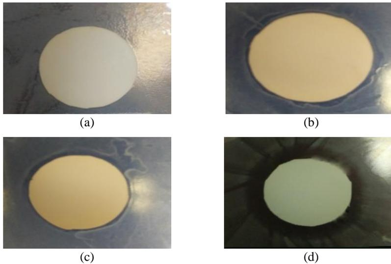
**Fig. 3. Results of membrane for antibacterial activity using agar diffusion method, (a) 7 wt.% PEG (Run 1) (No thickness of inhibition ring), (b) 5 wt.% zinc oxide (Run 4) (2-mm thickness of inhibition ring), (c) 5 wt.% eugenol (Run 8) (2-mm thickness of inhibition ring) and (d) 5 wt.% zinc oxide and 5 wt.% eugenol (Run 10) (6-mm thickness of inhibition ring).**
