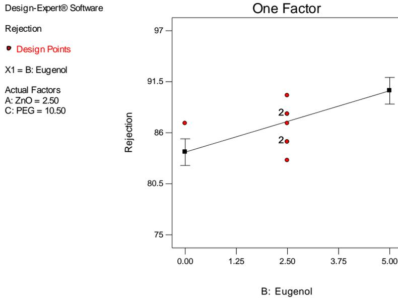
Fig. 9. Effect of eugenol on rejection properties of membrane.
