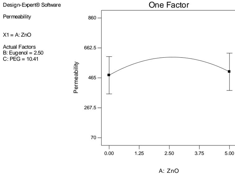
Fig. 6. Effect of zinc oxide on permeability of membrane.
