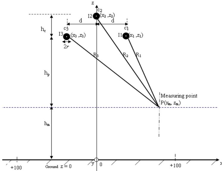
Fig. 4. Traverse section of a delta power line.
