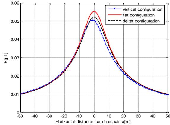
**Fig. 5. Comparison of the magnetic field intensity generated by different distribution power lines at the height of 1m from the ground.**
