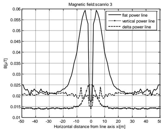
**Fig.10.** The distribution of the magnetic field intensity generated by a single distribution power line at the measuring situation *M3*.
