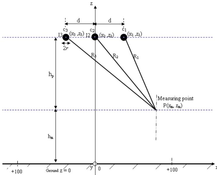
Fig. 3. Traverse section of a flat power line
