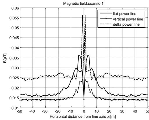
**Fig.8.** The distribution of the magnetic field intensity generated by a single distribution power line at the measuring situation *M1*.
