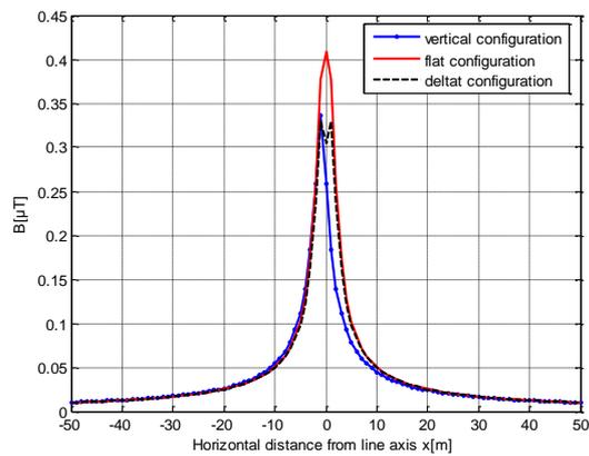
**Fig. 7. Comparison of the magnetic field intensity generated by different distribution power lines at the height of 9m from the ground.**
