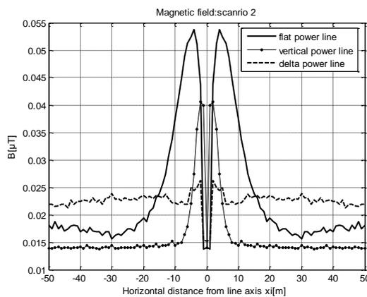
**Fig. 9.** The distribution of the magnetic field intensity generated by a single distribution power line at the measuring situation *M2*.
