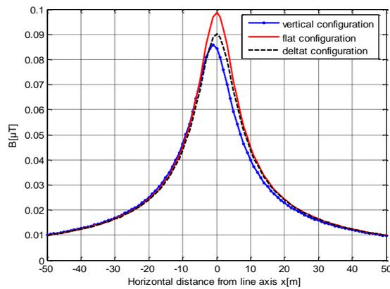
**Fig. 6. Comparison of the magnetic field intensity generated by different distribution power lines at the height of 5m from the ground.**
