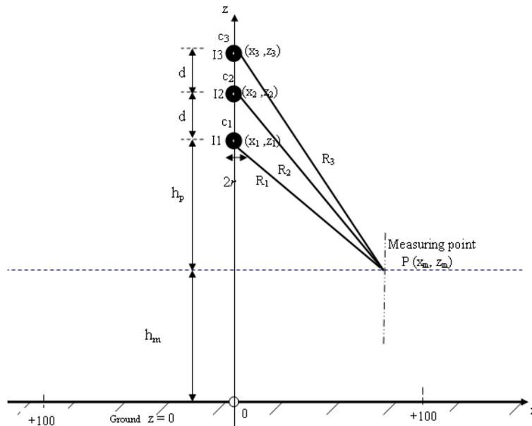
Fig. 2. Traverse section of a vertical power line.
