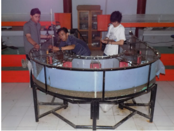
Fig. 2. Channels with bend of 180^\circ radius r_c = 0.75 meters.
