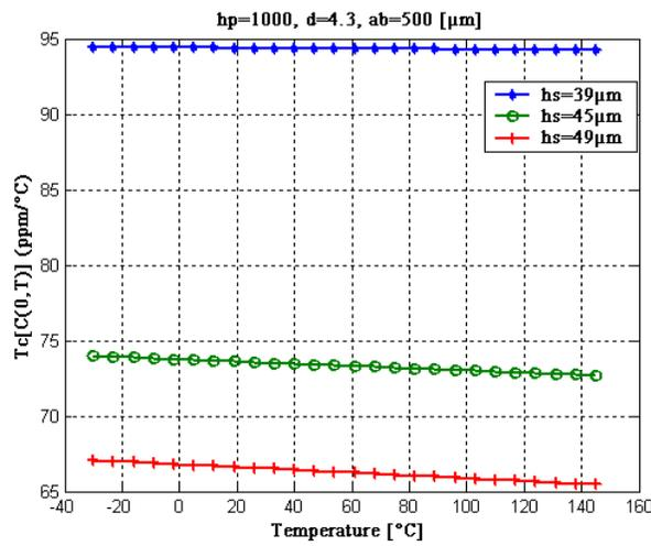
Fig. 6. Temperature Coefficient for Different Values of  $h_s$ .
