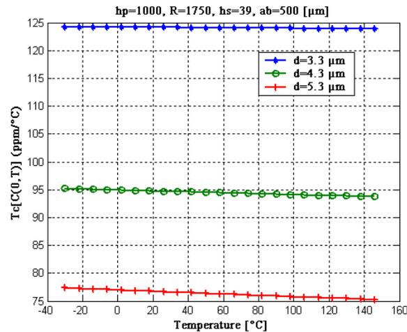
Fig. 8. Temperature Coefficient for Different Values of  $d$ .
