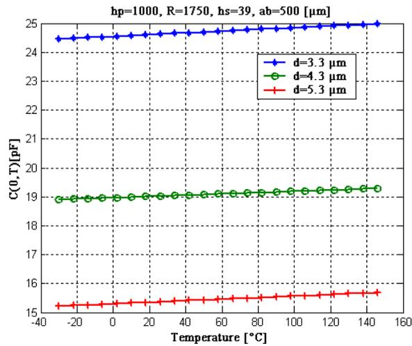
Fig. 7. Capacitance thermal variations for the different distance inter-electrode.
