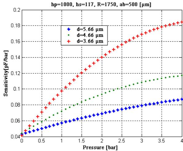
Fig. 15. Variation of sensitivity vs. pressure for the different distances inter-electrode.
