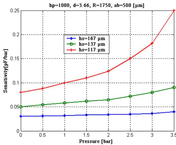
Fig. 13. Sensitivity variation vs. applied pressure  $P$ .
