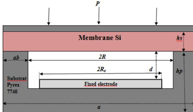
Fig. 1. Capacitive pressure sensor structure.
