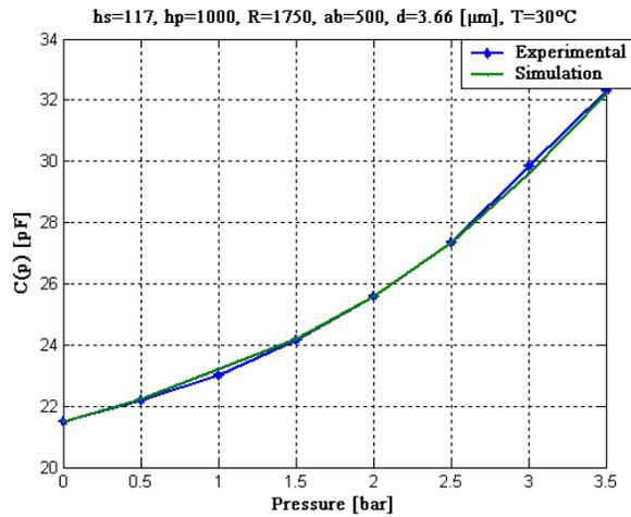
Fig. 2. Capacitance variation vs. applied pressure.
