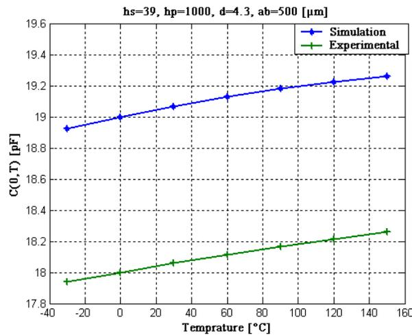
Fig. 3. Capacitance thermal variations.
