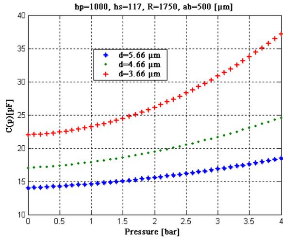
Fig. 14. Variation of capacitance vs. pressure for the different distances inter-electrode.
