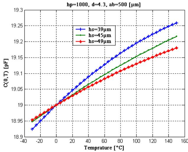
Fig. 5. Variation of the capacitance at rest as function of the temperature for different  $h_s$ .
