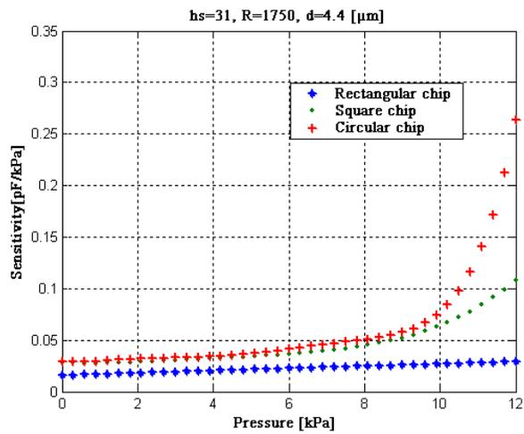
**Fig.11. Capacitance sensitivity variation vs. applied pressure for several membrane shapes.**
