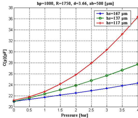
Fig. 12. Capacitance variation vs. applied pressure for several  $h_s$ .
