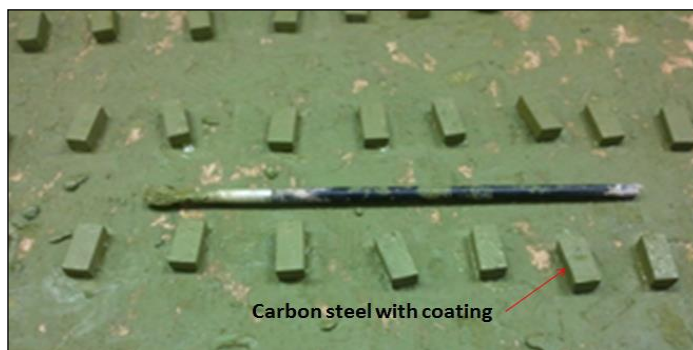
Fig. 1. Coating the steel coupons with prime coat.
