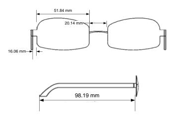
Fig. 2. The frame dimensions for female.
