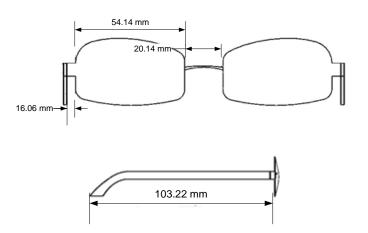
Fig. 3. The frame dimensions for male.
