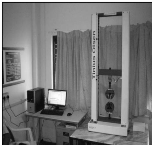
**Fig. 4. Tinius Olsen make universal testing machine.**
