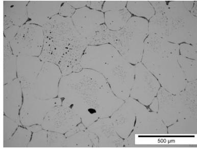
**Fig. 8. The microstructure of 5 hours aged at 400 °C of Cu-5Ni-5Sn alloy.**
