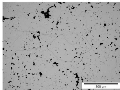
**Fig. 7. The microstructure of 4 hours aged at 400 °C of Cu-5Ni-5Sn alloy.**
