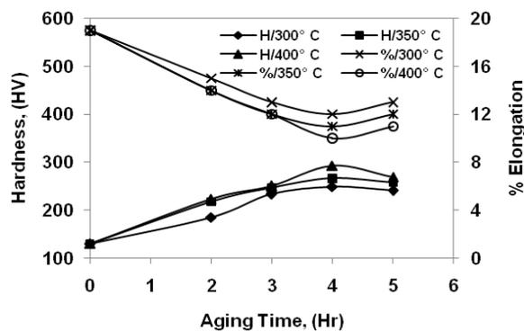
Fig. 11. Variation of hardness and % elongation of Cu-5Ni-5Sn alloy with aging time.
