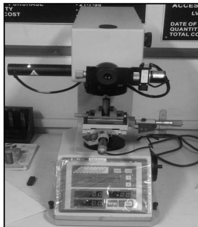
**Fig. 3. Mitutoyo make micro-hardness tester.**
