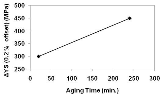
Fig. 15. Variation of yield stress with aging time, at 300 K tensile test temperature (Data of Kato and Schwartz [1]).
