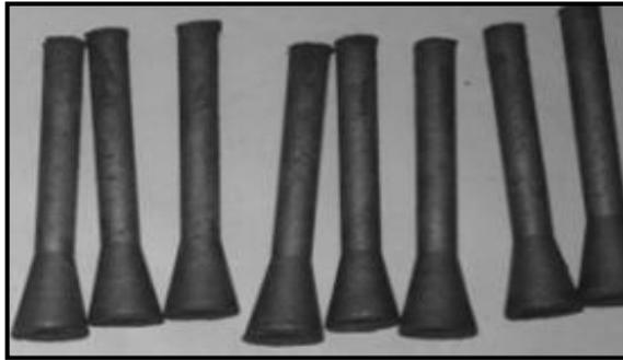
**Fig. 2. Cast rods of Cu-5Ni-5Sn alloy.**
