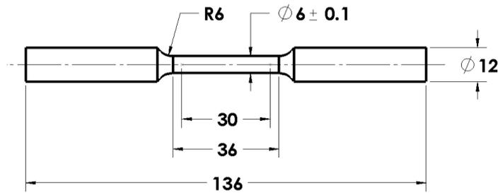
**Fig. 5. Dimensions of the tensile test specimen.**
