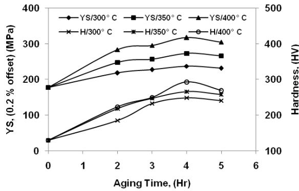
**Fig. 12. Variation of yield stress and hardness of Cu-5Ni-5Sn alloy with aging temperature and time.**
