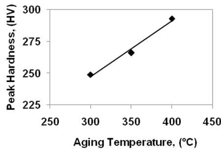
Fig. 10. The variation of peak hardness of Cu-5Ni-5Sn alloy with aging temperature.
