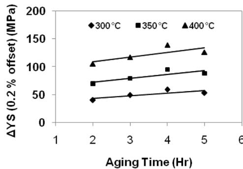
Fig. 14. Variation of incremental yield stress with aging temperature and time.
