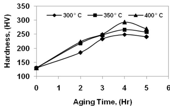
**Fig. 9. Variation of hardness of Cu-5Ni-5Sn alloy with aging temperatures and time.**
