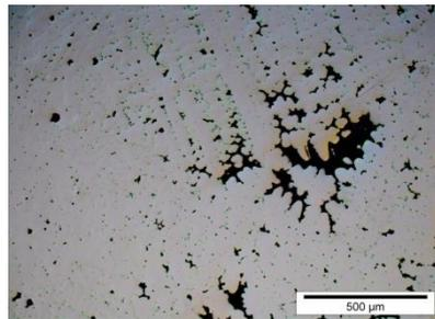
**Fig. 6. As-cast microstructure of Cu-5Ni-5Sn alloy.**
