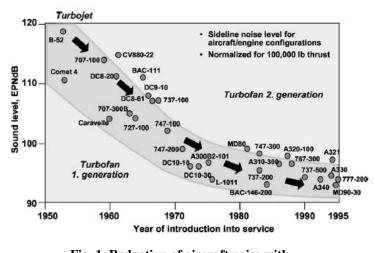
Fig. 1. Reduction of aircraft noise with to respect the year of entry into service [12].
