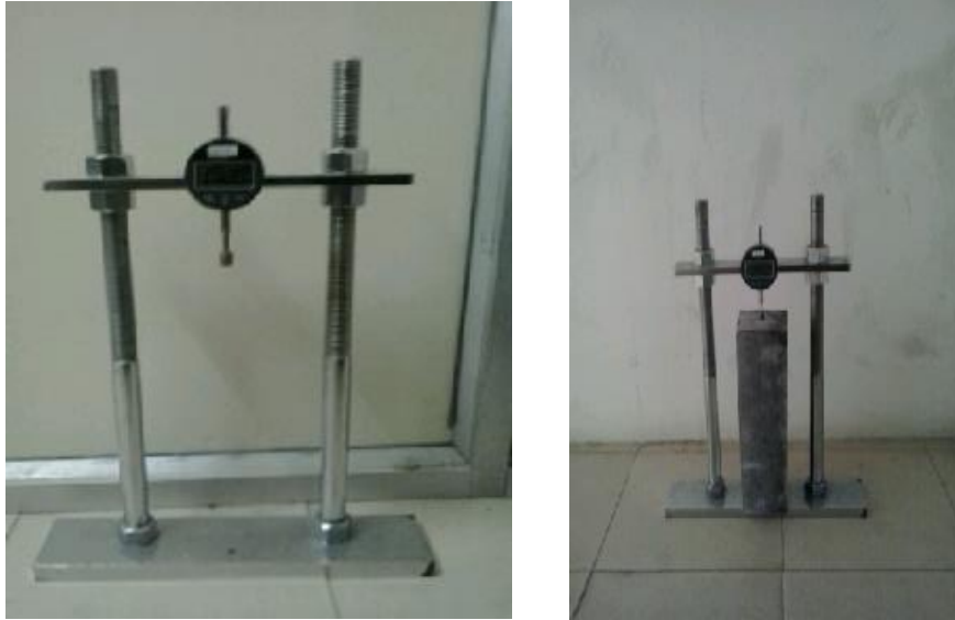
Fig. 1. Drying shrinkage apparatus and testing of the specimen.
