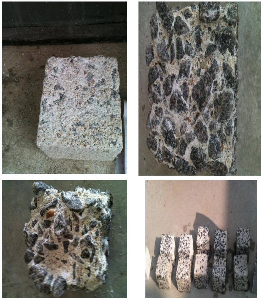
Fig. 2. Deterioration of concrete specimens due to acid attack.
