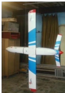
Fig. 10. Bifilar torsional pendulum method.
