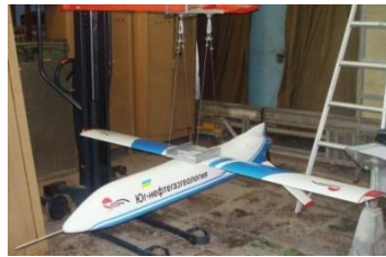
Fig. 9. Physical pendulum method.
