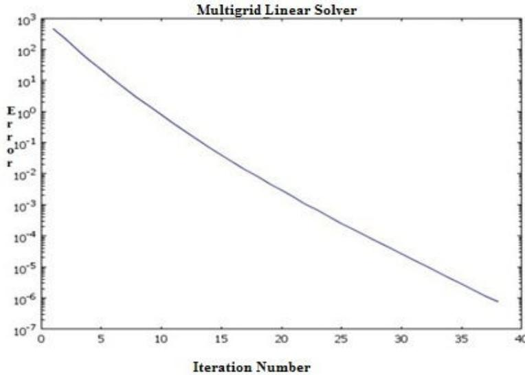
Fig. 3. Error convergence plot using geometric multigrid linear solver.
