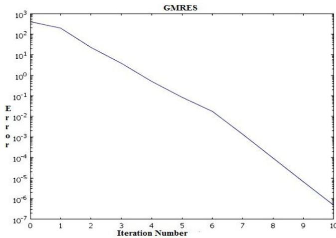
**Fig. 2. Error convergence plot using GMRES solver.**
