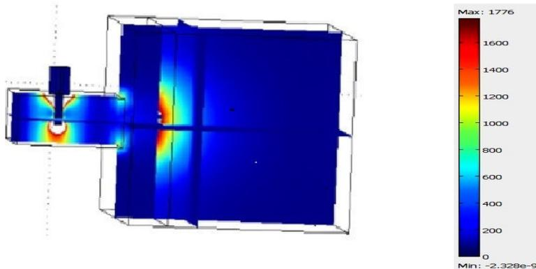
**Fig. 6. SAR heat distribution in the muscle phantom.**
