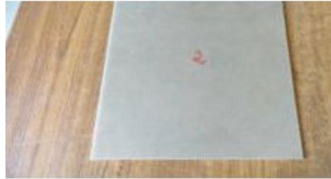
Fig. 2. Specimen - II 60% epoxy and 40% E-fiberglass.
