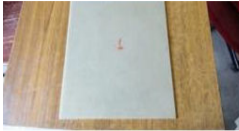
Fig. 1. Specimen - I 40% epoxy and 60% E-fiberglass.
