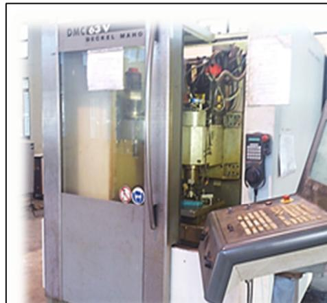
**Fig. 2. Vertical Machining Centre used for Experiment.**
