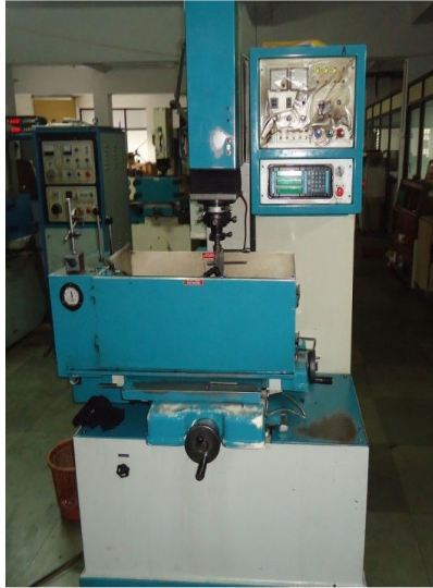
Fig. 1. Electronica ZNC die sinker machine. Fig. 2. Machined test specimen.
