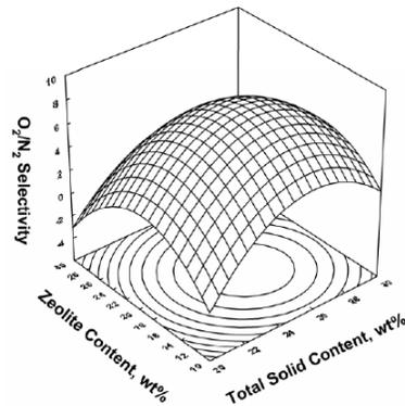
**Fig. 5. The surface and contour plot of the effect of total solid content and zeolite content on O<sub>2</sub>/N<sub>2</sub> selectivity at constant level of polymer blending composition = 25 wt%.**
