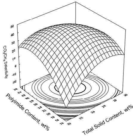
**Fig. 3. The surface and contour plot of the effect of total solid content and polymer blending composition on  $\text{CO}_2/\text{CH}_4$  selectivity at constant level of zeolite loading = 20 wt%.**
