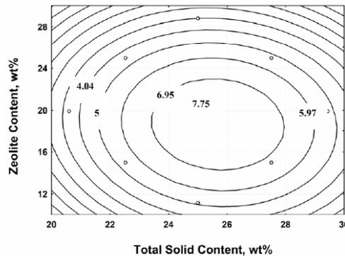
**Fig. 6. The contour plot of the effect of total solid content and zeolite content on O<sub>2</sub>/N<sub>2</sub> selectivity at constant level of polymer blending composition = 25 wt%.**
