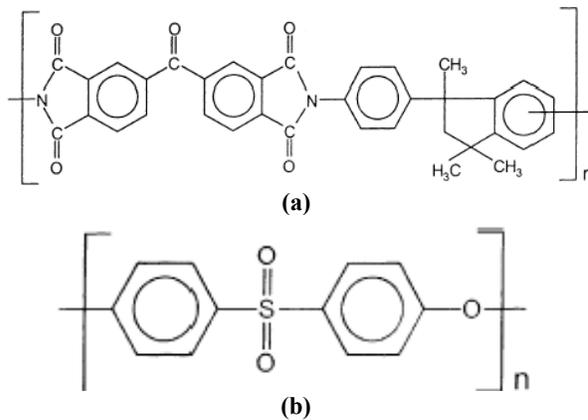
**Fig. 1. Chemical structure of (a) Polyimide and (b) Polyethersulfone.**
