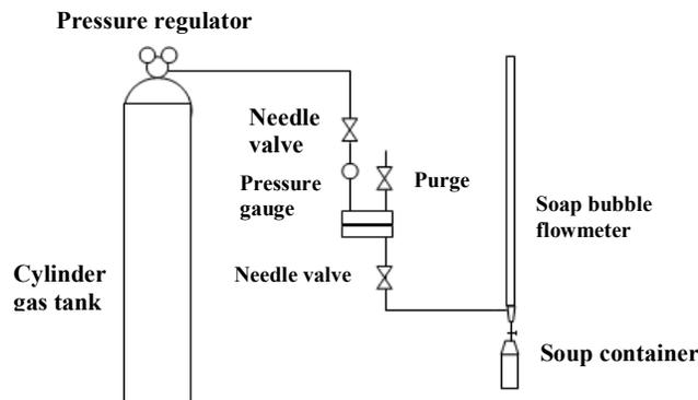
**Fig. 2. Flat sheet membrane gas permeation measurement set up.**
