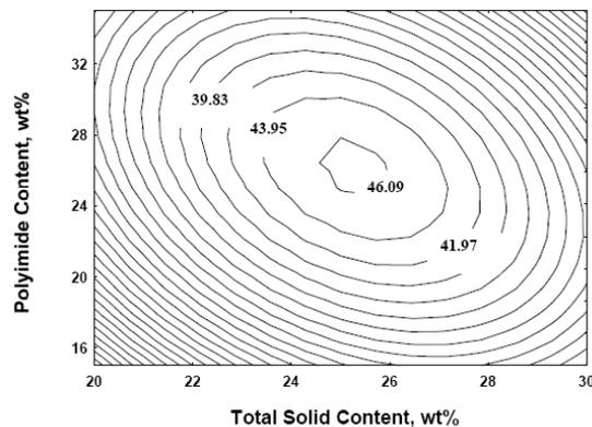
**Fig. 4. The contour plot of the effect of total solid content and polymer blending composition on  $\text{CO}_2/\text{CH}_4$  selectivity at constant level of zeolite loading = 20 wt%.**
