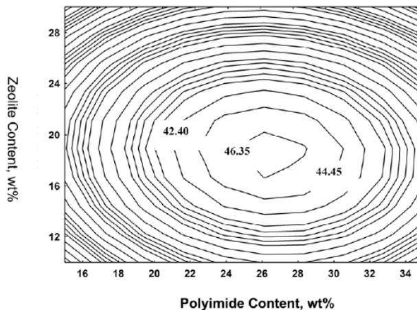
Fig. 8. The contour plot of the effect of polymer blending composition and zeolite content on  $\text{CO}_2/\text{CH}_4$  selectivity at constant level of total solid content = 25 wt%.
