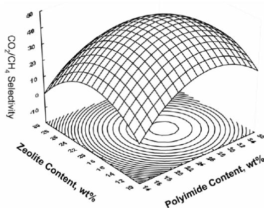
Fig. 7. The surface and contour plot of the effect of polymer blending composition and zeolite content on  $\text{CO}_2/\text{CH}_4$  selectivity at constant level of total solid content = 25 wt%.
