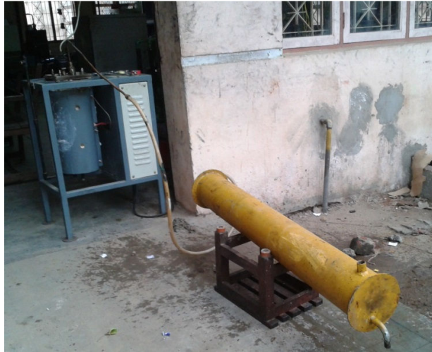
Fig. 1. Photographic view of the catalytic thermal reactor with condenser.
