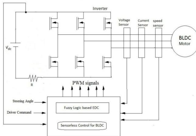
**Fig. 2. Fuzzy logic based electronic differential controller.**
