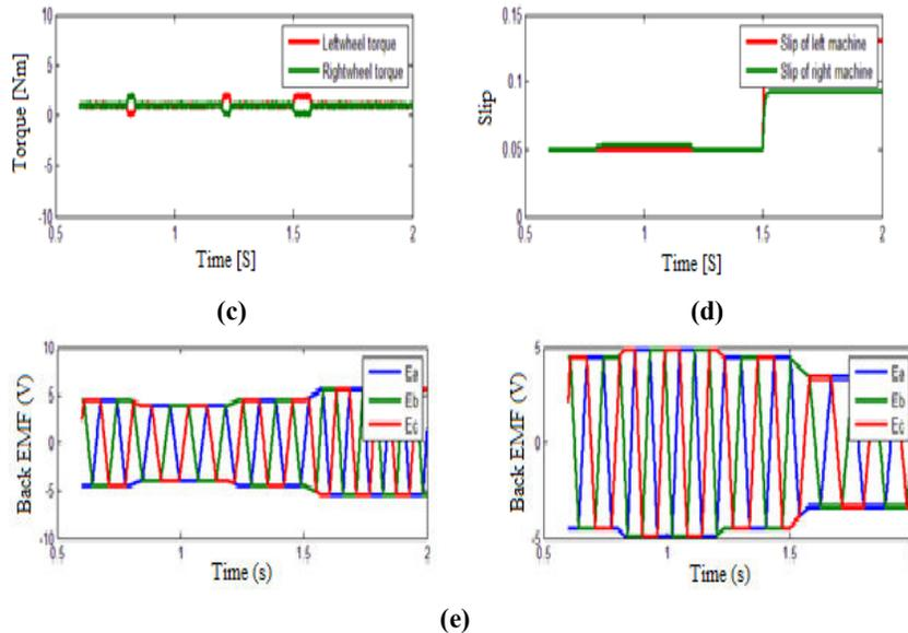
**Fig. 6. The performance of the Fuzzy based EDC with third harmonics voltage integration. (a) Speed waveform of left and right side motor (b) Current wave form for left and right side motor (c) Torque wave form for left and right side motor (d) Slip rate waveform for left and right side motor (e) Back EMF wave form of left and right side motor.**
