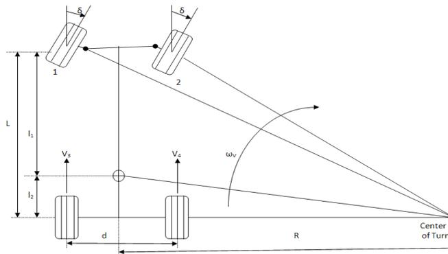
**Fig. 1. Vehicle structure.**
