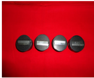
Fig. 4. Moulded sample for microscopic examination.
