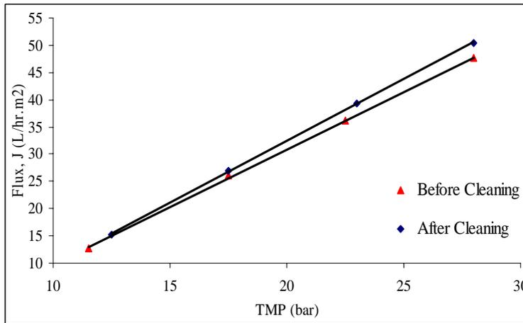
Fig. 2. Permeate flux before and after chemical cleaning.
