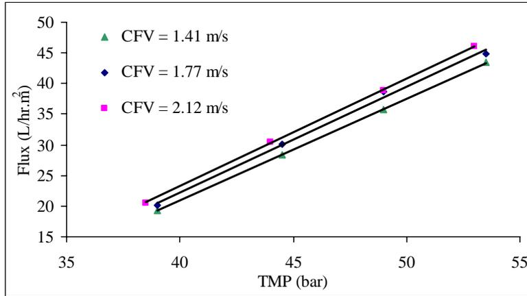
**Fig. 3. Effect of CFV at constant temperature of 35°C on permeate flux.**
