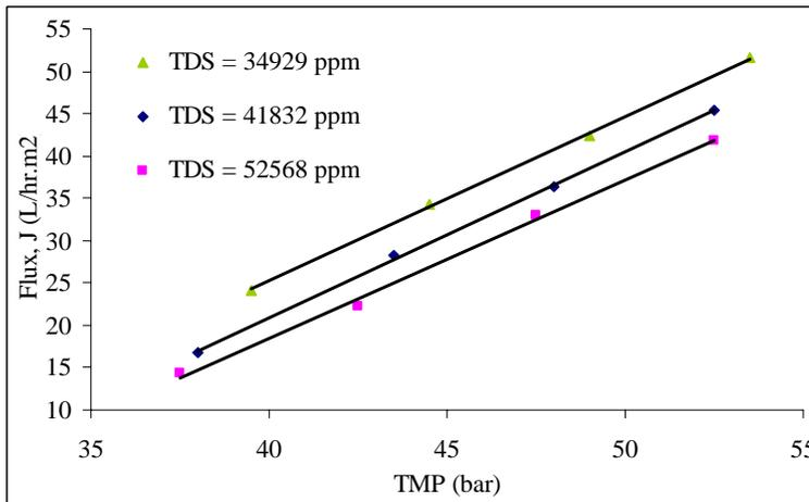
Fig. 5. Effect of feed concentration on the permeate flux.
