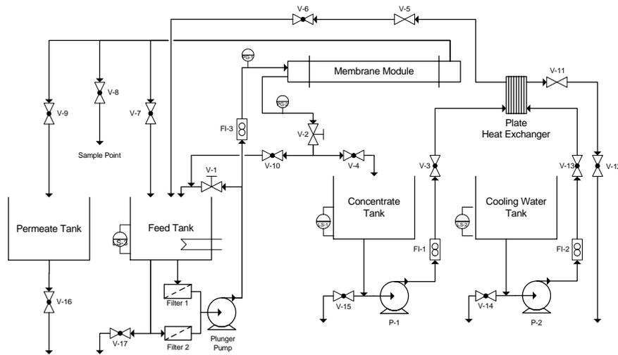
**Fig. 1. Schematic diagram of RO system**
