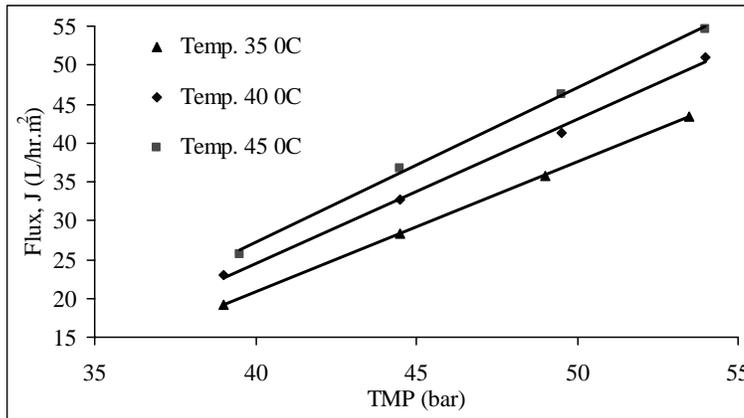
Fig. 4. Effect of feed temperature at constant CFV of 1.41 m/s on permeate flux.
