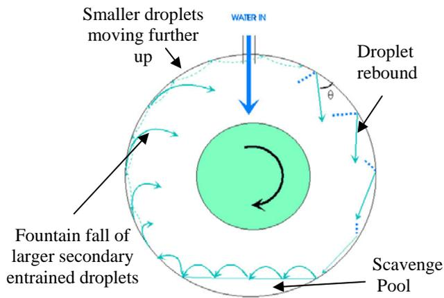
**Fig.4. Flow patterns from the stationary casing.**
