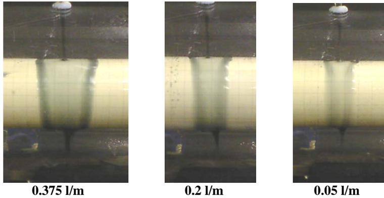
Fig.6. Film spread and ligament effects on the stationary shaft.
