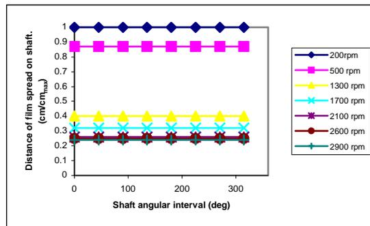
**Fig.11. Film spread effects at each angular location for 0.375 l/m for various rotor speeds**
