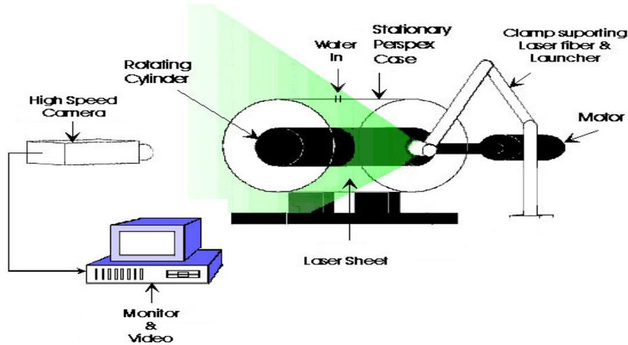
Fig. 1. Laser sheet visualisation set-up.
