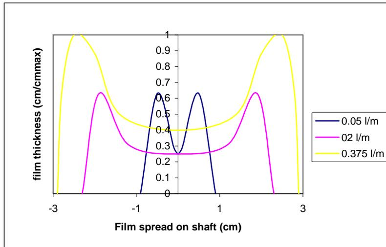
**Fig.8. Variation of film thickness across the film band at 90° location.**
