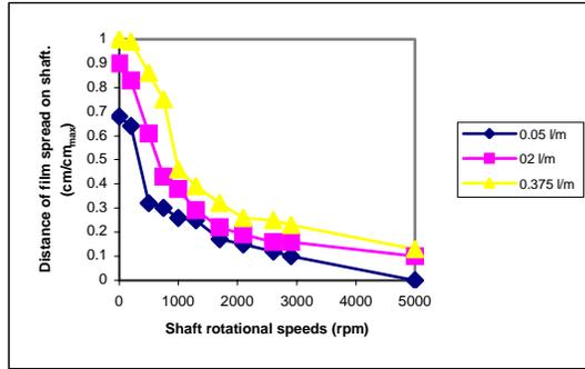
Fig.12. Variation of (full) film spread for increase rotor speeds at 0°.
