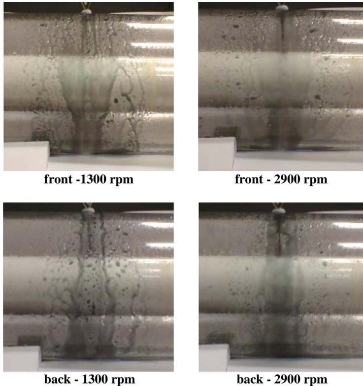
**Fig.20. Film on the surface of the Perspex casing for 0.375 l/m.**
