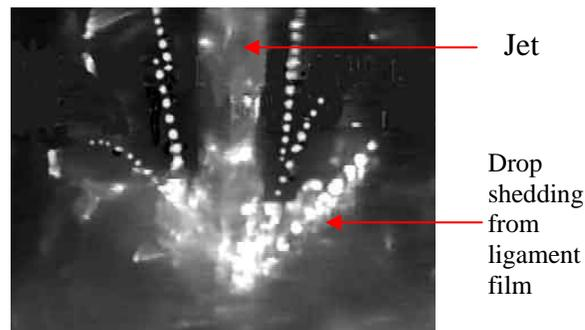
**Fig.17. Drop shedding effects from the ligament film behind the jet.**
