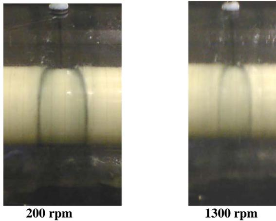
**Fig.15. The film spread effects on the shaft for various rotor speeds (0.375 l/m).**
