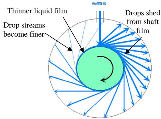
**Fig.3. Flow patterns from the shaft region.**
