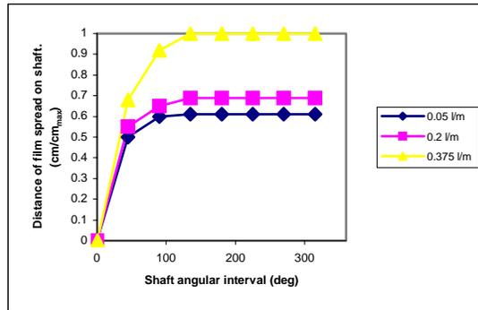
**Fig.14. Variation of parabolic effects at 200 rpm for various flow rates.**
