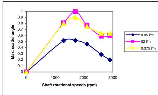
**Fig.19. Variation of scatter angles impinging on casing surface.**
