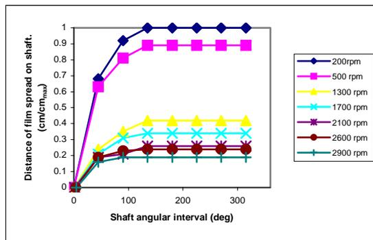
Fig.13. Variation of parabolic cone for 0.375 l/m for various rotor speeds.
