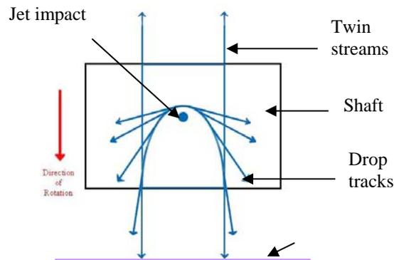
**Fig. 16. Drop shedding from ligament film from the rotating shaft.**
