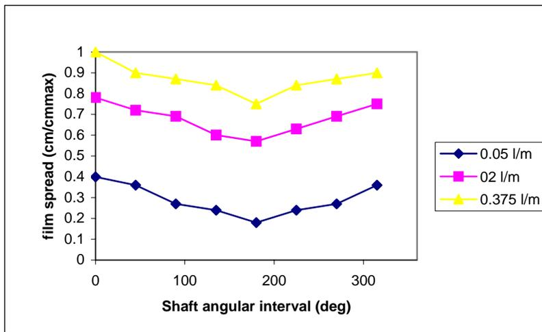
Fig.7. Variation of film spread at each angular location on the stationary shaft.
