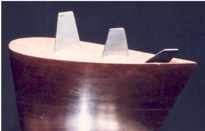
**Fig.2. NACA0012 wing fitted with three wing tip sails.**
