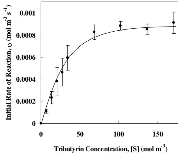
**Fig.1. The change of initial rate of reaction at different initial substrate concentration, [S]**
