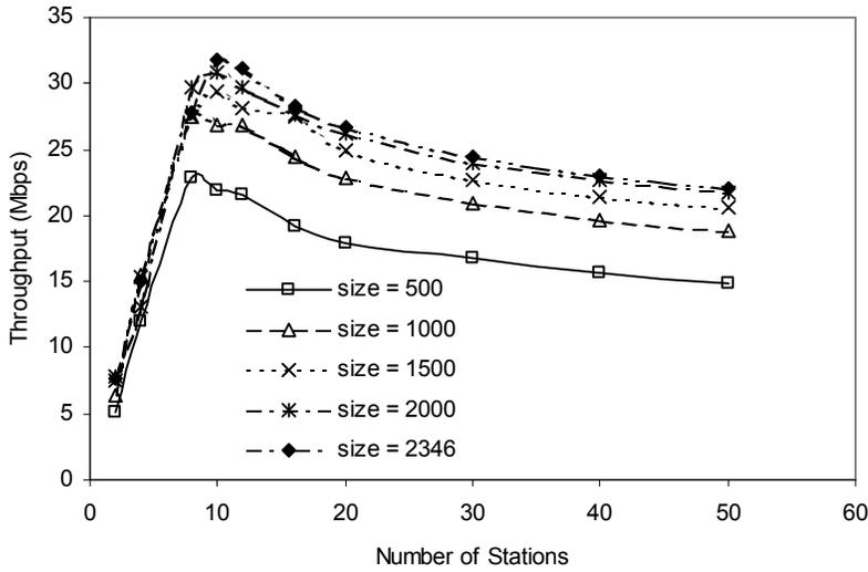
**Fig. 4. Throughput versus the number of stations for different frame sizes**
