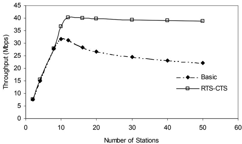
**Fig. 8. Throughput versus the number of stations for both access schemes**
