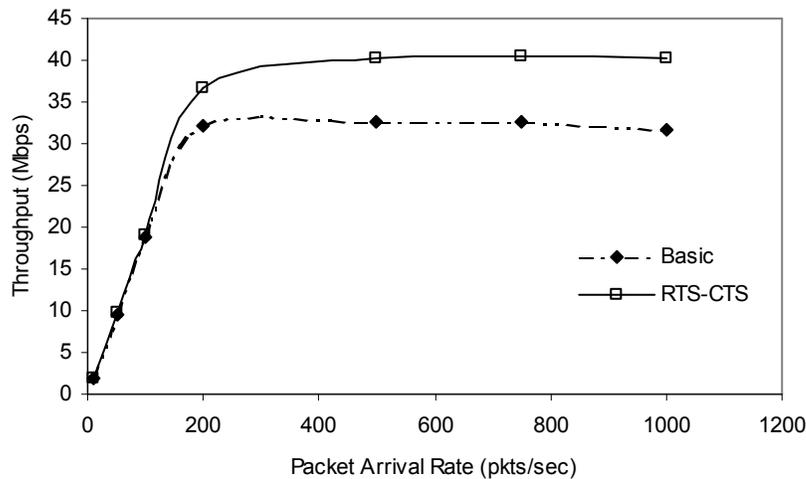
**Fig. 6. Throughput versus the packet arrival rate for both access schemes**
