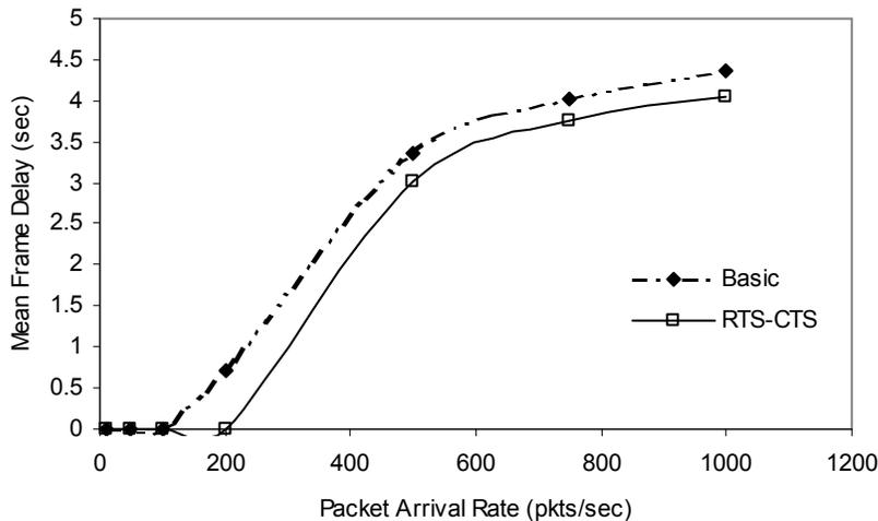
**Fig. 5. Mean frame transmission delay versus the packet arrival rate for both access schemes**
