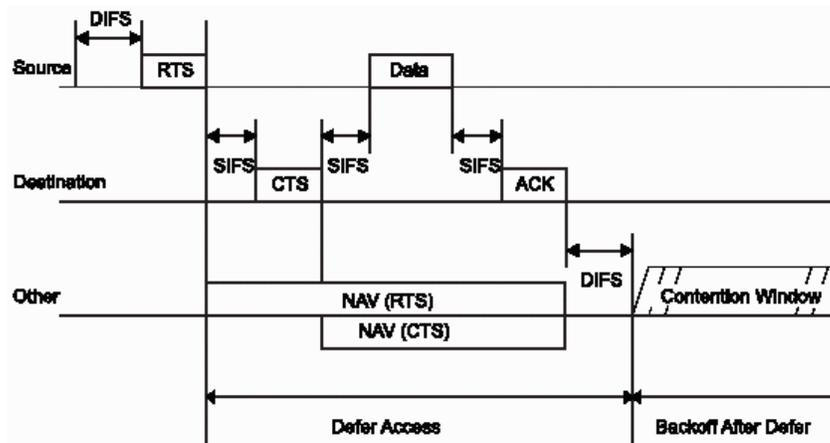
Fig.1. The RTS/CTS access mechanism (adapted from [1])
