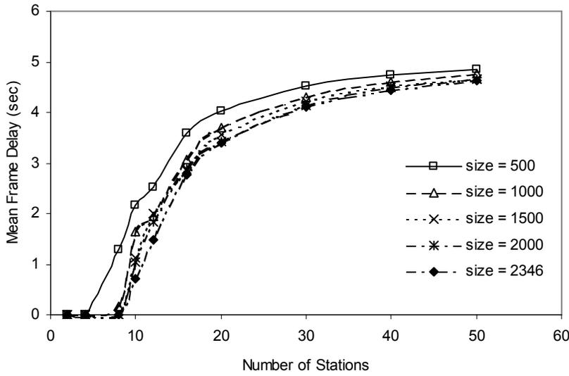
**Fig. 3. Mean frame transmission delay versus the number of stations for different frame sizes.**
