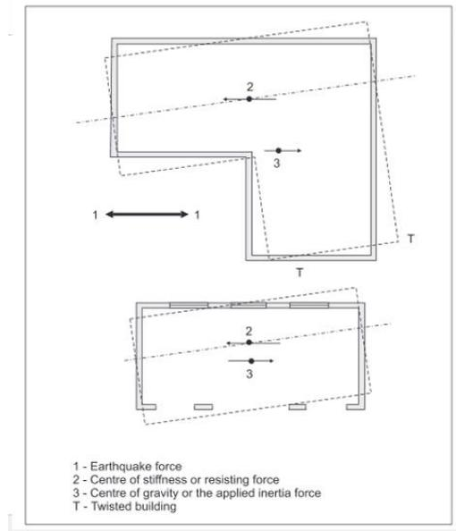
**Fig. 6. Asymmetrical plan (design obtained from national information center of earthquake engineering).**
