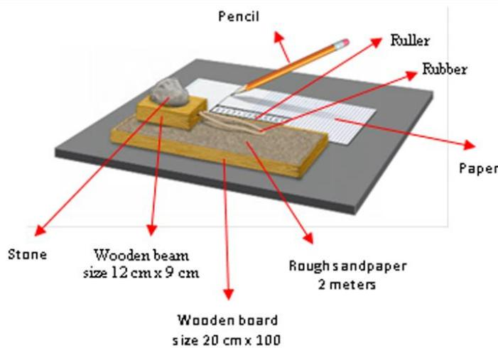
**Fig. 2. The design of earthquake machine.**
