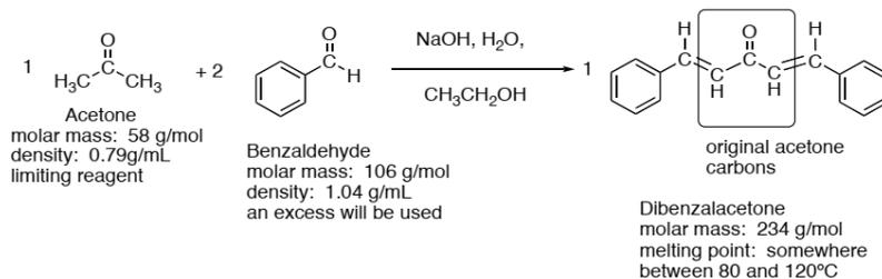
**Fig. 2. Synthesis reaction of Dibenzalacetone [10].**
