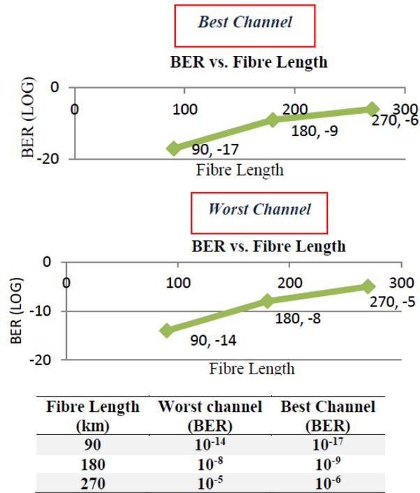
Fig. 6. BER Values of 8 Channel Duobinary (Bit rate~ 40 Gb/s).
