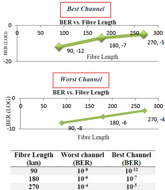
Fig. 7. BER Values of 16 Channel Duobinary (Bit rate~ 40 Gb/s).
