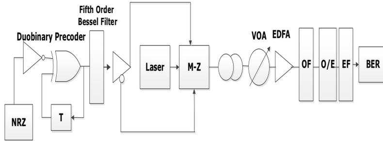
Fig. 1. Transmitter set-up of Duobinary modulation.
