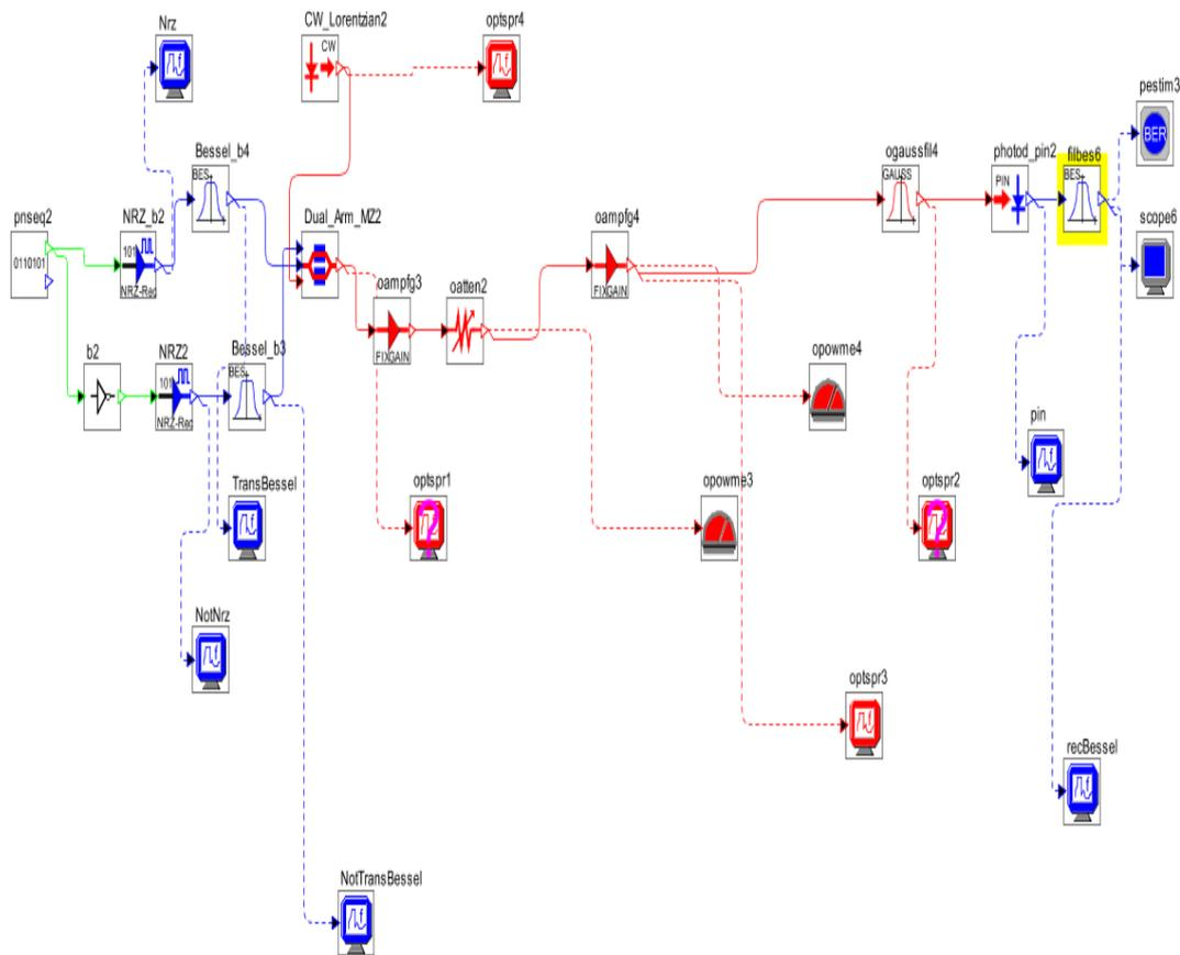
Fig. 3. Duobinary transmitter and receiver set-up in single mode fibre communication link.
