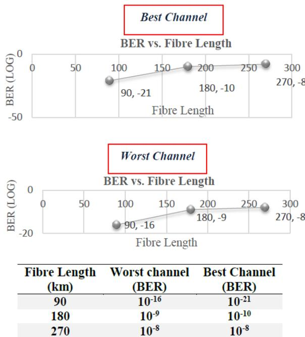
Fig. 5. BER Values of 4 Channel Duobinary (Bit rate~ 40 Gb/s).
