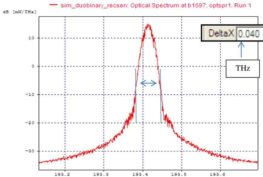
**Fig. 4. Optical Spectrum for RZ-OOK (Bit Rate~ 40 Gb/s).**
