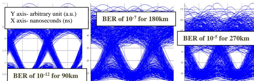
Fig. 8. Eye diagrams for 16 Channel WDM of Duobinary modulation format.
