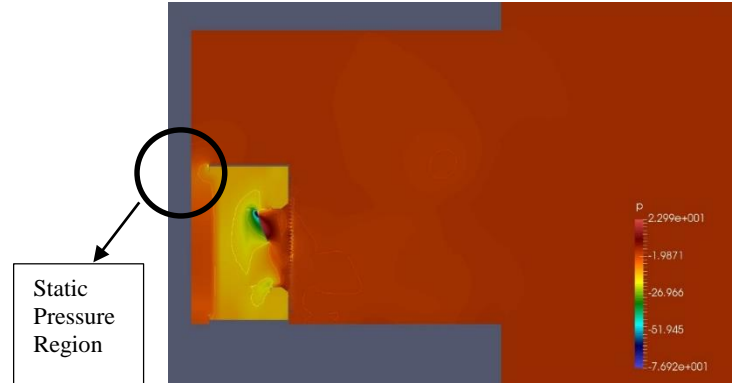
Fig. 13. Static pressure behind the outdoor unit.
