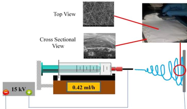
**Fig. 1. Schematic of electrospinning system.**
