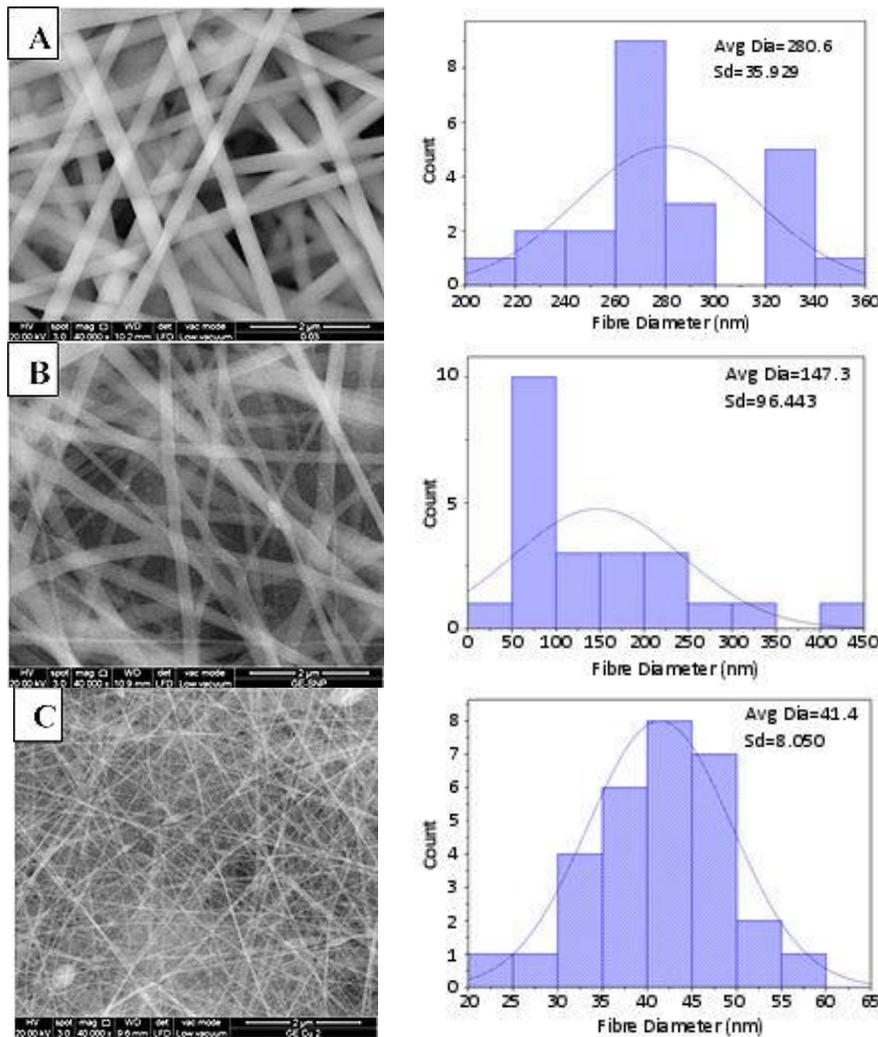
**Fig. 3. SEM micrograph of the Ge-espun nanofibers and diameter distribution of (A) neat Ge-espun (B) Ag/Ge-espun (C) Cu/Ge-espun**
