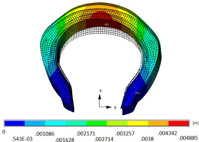
**Fig. 10. Vertical displacement deformation (x-direction): initial deformation (wire frame) and final deformation at pressure 230 kPa.**
