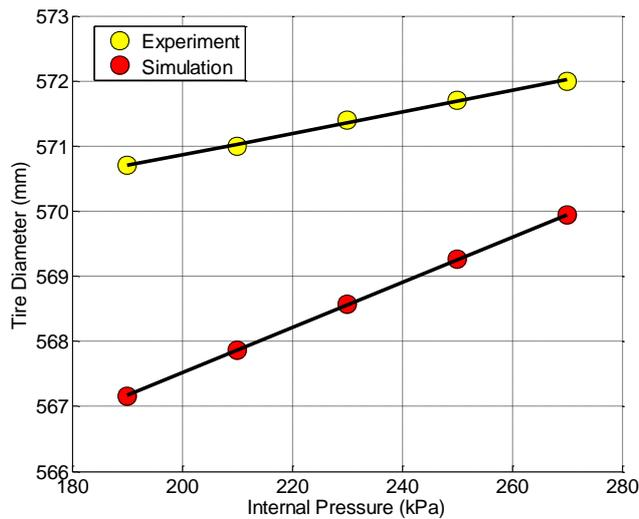
**Fig. 9. Comparisons of experimental tire and simulation results.**
