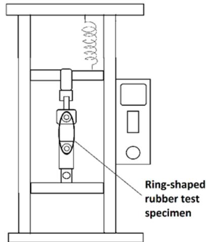
**Fig. 2. Ring testing machine.**
