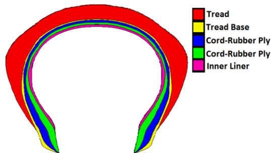
**Fig. 5. 3D Model for the bias two-wheel tire.**
