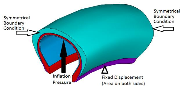
**Fig. 6. Boundary condition of 3D tire model (20-degree).**
