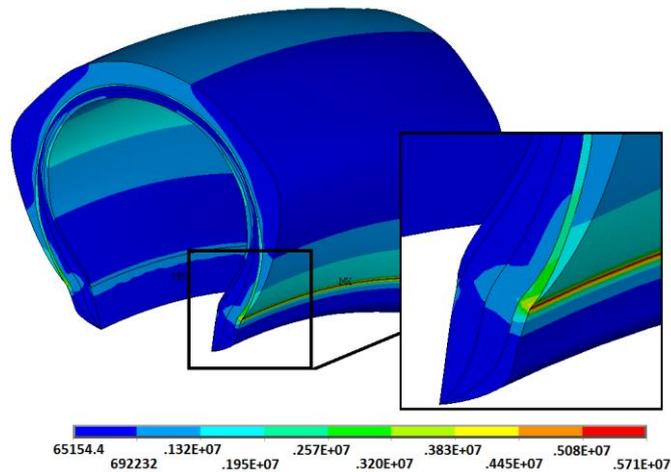
**Fig. 13. Von-Mises stress of the bias tire (MPa).**
