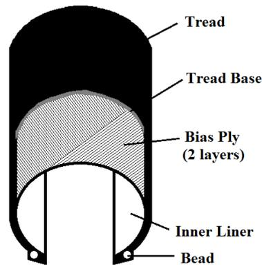
**Fig. 1. Components of bias tire.**
