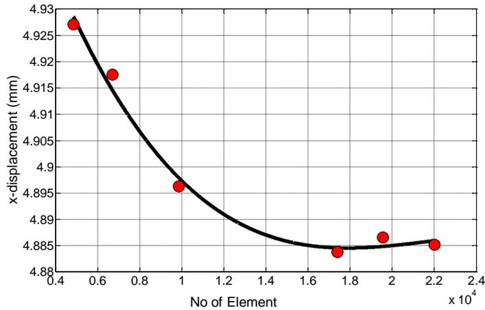
Fig. 7. Convergence test using x-displacement at various element numbers.
