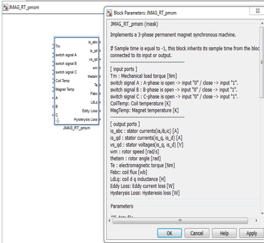
Fig. 4. JMAG-RT in SIMULINK.
