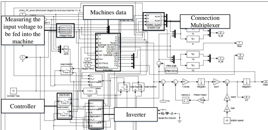
Fig. 5. JMAG RT circuitry in SIMULINK.
