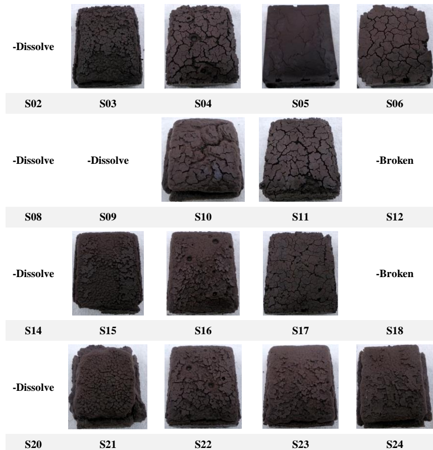
Fig. 2. Samples condition after the water absorption test.
