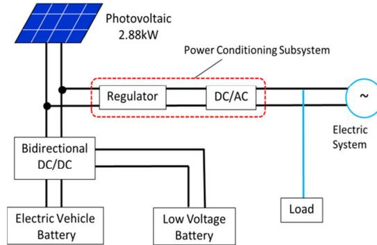
**Fig. 6. Outline of the Power Supply System Model.**
