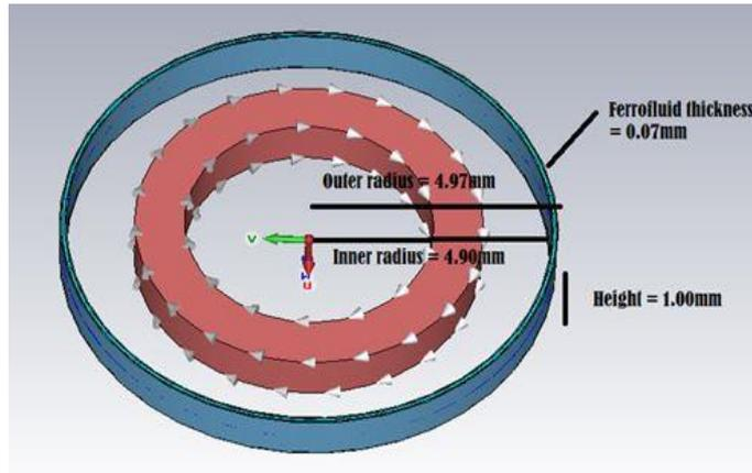
**Fig. 1. The design for aqueous magnetic material.**
