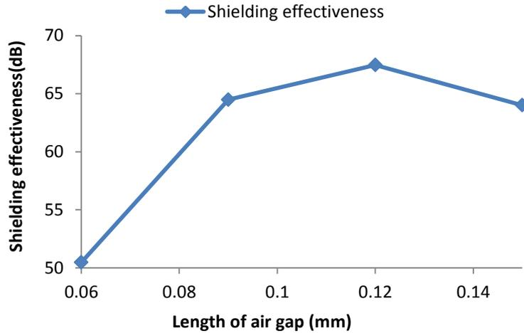
**Fig. 6. Shielding effectiveness with different length of air gap.**
