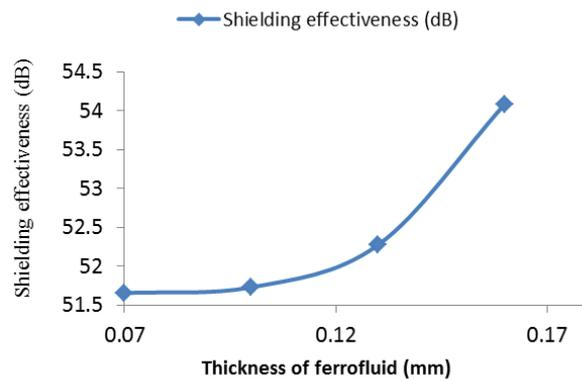
**Fig. 5.** Shielding effectiveness of materials with different thickness of ferrofluid.
