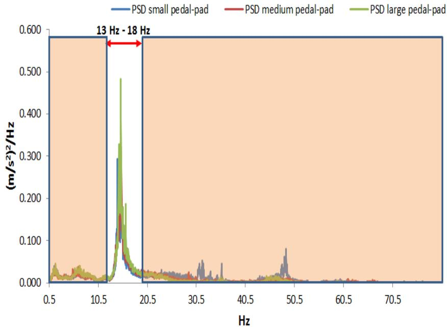
**Fig. 3. PSD between the frequency ranges of 0.5 Hz to 80 Hz for the three different sizes of pedal-pad**
