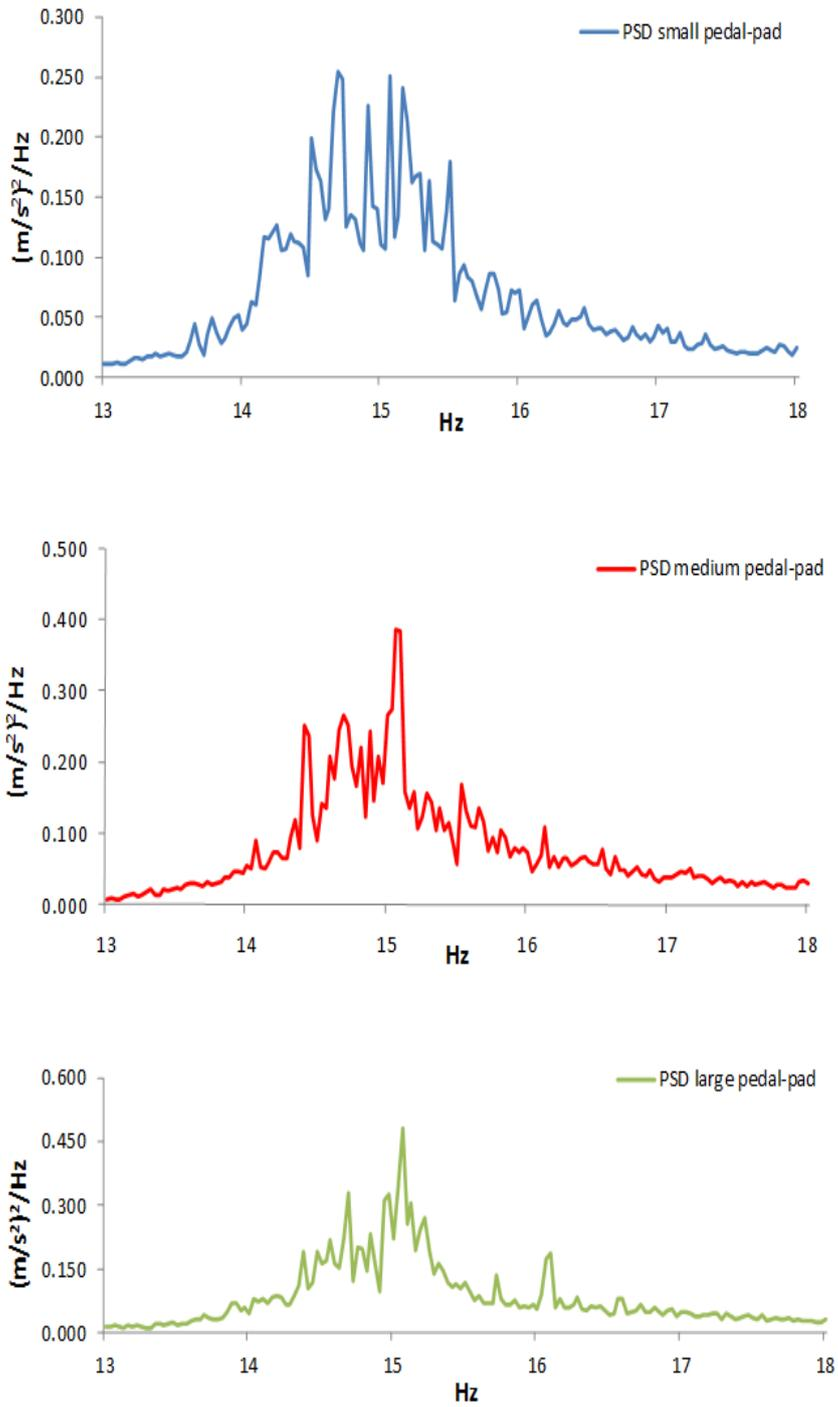
**Fig. 4.** PSD between the frequency range of 13 Hz to 18 Hz for (a) Small size pedal-pad, (b) Medium size pedal-pad, and (c) Large size pedal-pad
