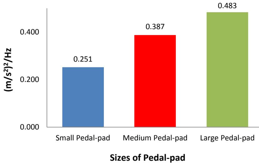
**Fig. 5. Peak value at resonance frequency 15 Hz for the three different sizes of pedal-pad**
