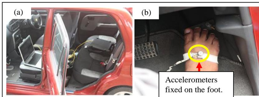
**Fig. 2. The method of affixing the (a) equipment and (b) accelerometer on the foot**
