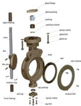
Figure 4.1 Butterfly Valve’s Component
