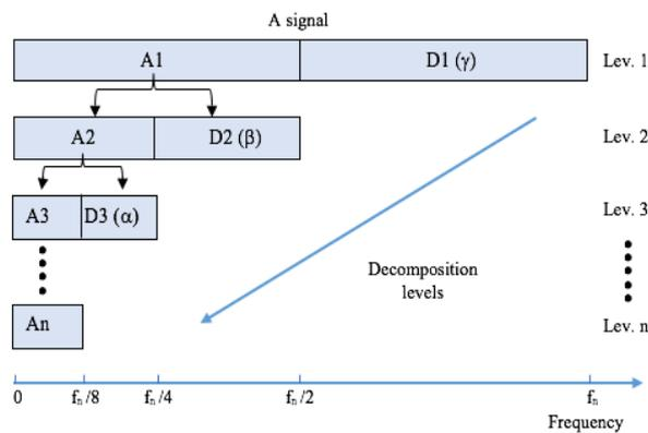
Fig. 2. Operation of EEG analysis using the DWT.
