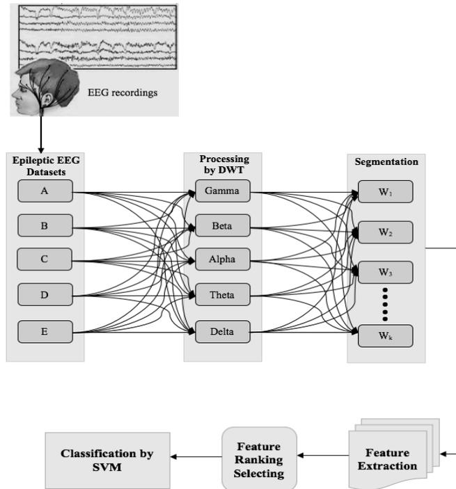
Fig. 1. Block diagram of the suggested method for EEG analysis and classification.
