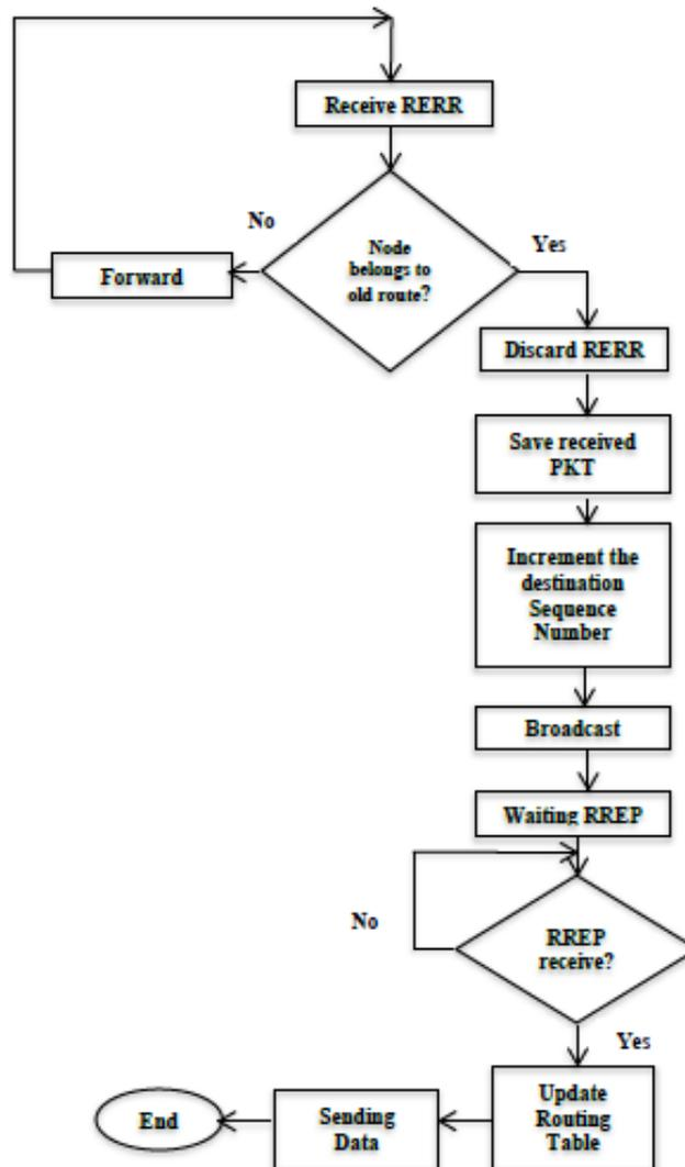
Fig. 2. UAODV Route maintenance phase performed by the upstream node to the link breakage.
