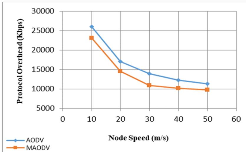
Fig. 4(e). Protocol overhead versus node speed.
