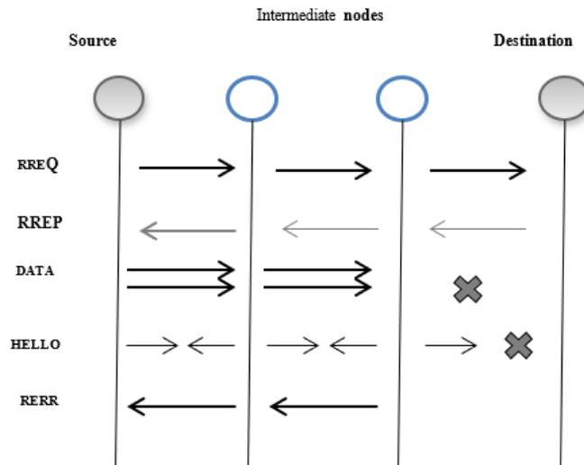
Fig. 1. AODV operation mechanism.
