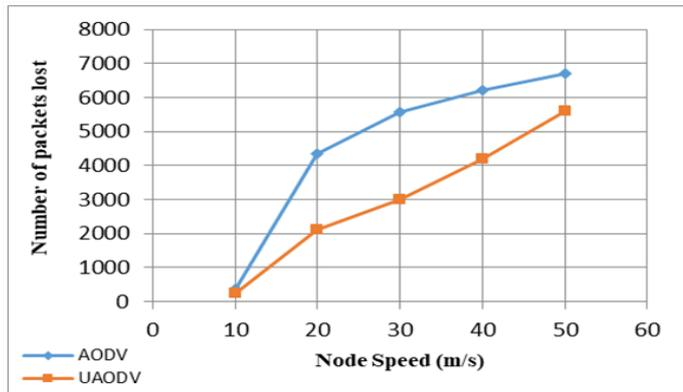
Fig. 4(b). Lost packets versus node speed.
