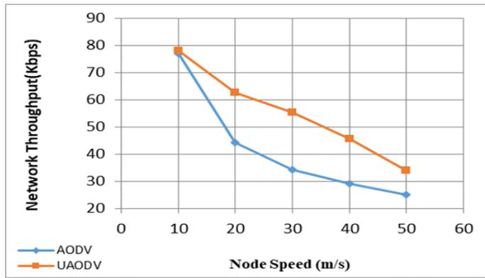
Fig. 4(a). Network throughput versus node speed.
