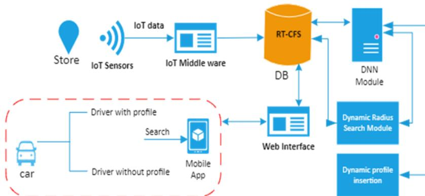
Fig. 3. high level diagram for the proposed systems.
