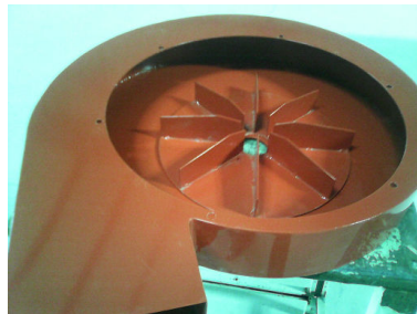
Fig. 14. Experimental model of blower and fan assembly.
